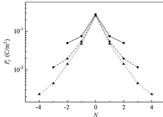
**Figure 2** The polarization profiles for  $(\text{KNbO}_3)_1(\text{KTaO}_3)_n$  superlattices with  $n = 3, 5,$  and  $7$ . The number  $N = 0$  corresponds to the  $\text{KNbO}_3$  layer.**Table 3** The energy difference between ferroelectrically and antiferroelectrically ordered structures in  $[(\text{KNbO}_3)_1(\text{KTaO}_3)_n]_2$  superlattices (per Nb atom).
