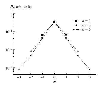
**Fig. 4.** The polarization distribution between the layers in the ground-state structure of  $(BaTiO_3)_1(BaZrO_3)_n$  superlattices with n = 1, 3, and 5. The layer number N = 0 corresponds to the BaTiO<sub>3</sub> layer.
