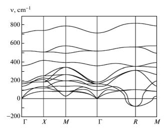
**Fig. 1.** Phonon spectrum of the BaZrO<sub>3</sub> crystal in the cubic phase.
