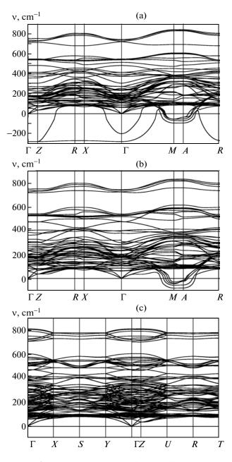
Fig. 2. Phonon spectra of the free-standing  $(BaTiO_3)_1(BaZrO_3)_3$  superlattice in (a) *P4/mmm*, (b) *Amm2*, and (c) *Pmc2*<sub>1</sub> phases.
