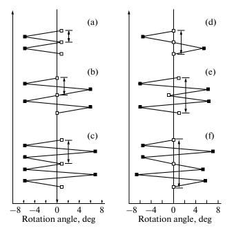
**Fig. 3.** Octahedra rotation angles in the ground state of  $(BaTiO_3)_1(BaZrO_3)_n$  superlattices corresponding to the phonon condensation at points (a–c) *M* and (d–f) *A*. (a, d) n = 1 (L = 2), (b, e) n = 2 (L = 3), (c, f) n = 3 (L = 4). BaTiO<sub>3</sub> and BaZrO<sub>3</sub> layers are denoted by open and filled squares, respectively. Vertical lines with arrows indicate the physical periods of the resulting structures.
